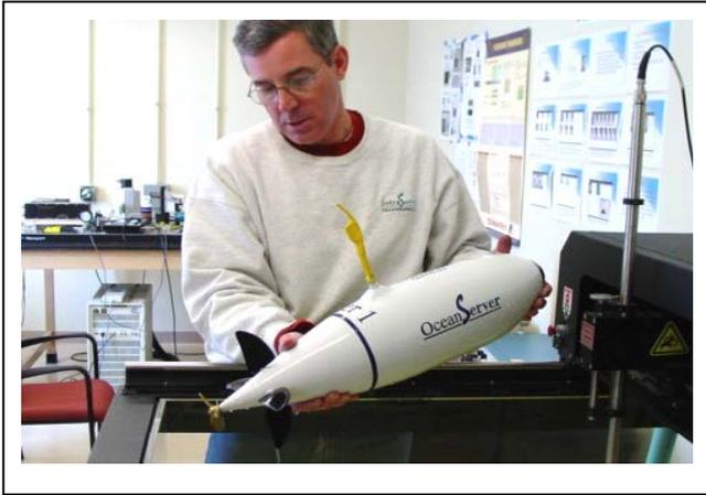
Photo of the original Iver 1 vehicle during tank testing
