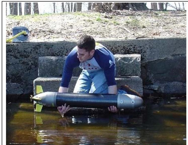
Photo of Iver 2 prototype during free-water testing
