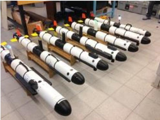
two new Iver3-450 Nano AUVs. The Iver3 Nano AUVs represent a new class of very small lightweight AUVs weighing less than 39 Lbs with modern chirp based sonar. Two new Iver3-580 systems have already been delivered to the Navy EOD Group and the other 2 will be delivered within the next few months to the The Naval Oceanography Special Warfare Center (NOSWC).
